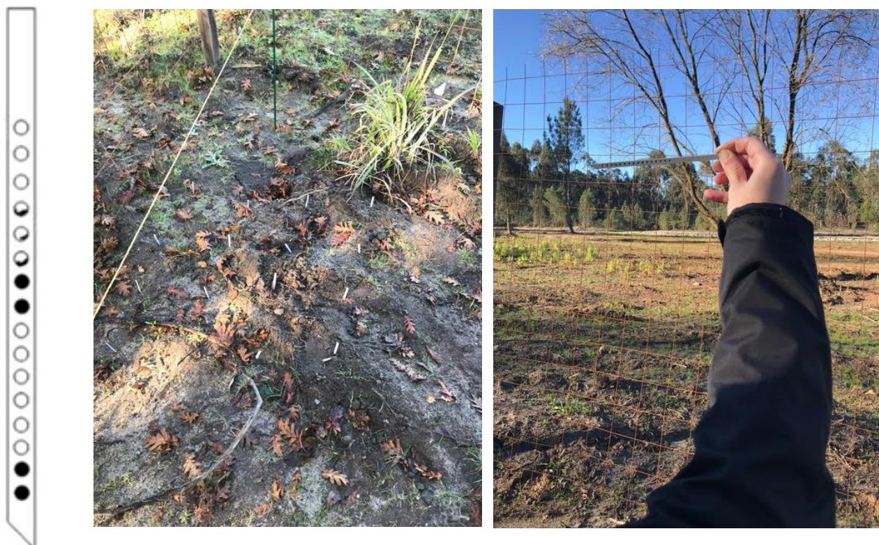
Figure NS8. 29 – Scheme of a bait lamina with empty (white circles), partially empty (partially dark circles) and filled (full dark circles) holes (left draw), a group of 16 bait lamina sticks inserted into the soil (left photo) and a sampled bait lamina (right photo).
